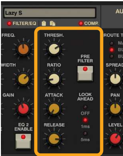
The Compressor section
